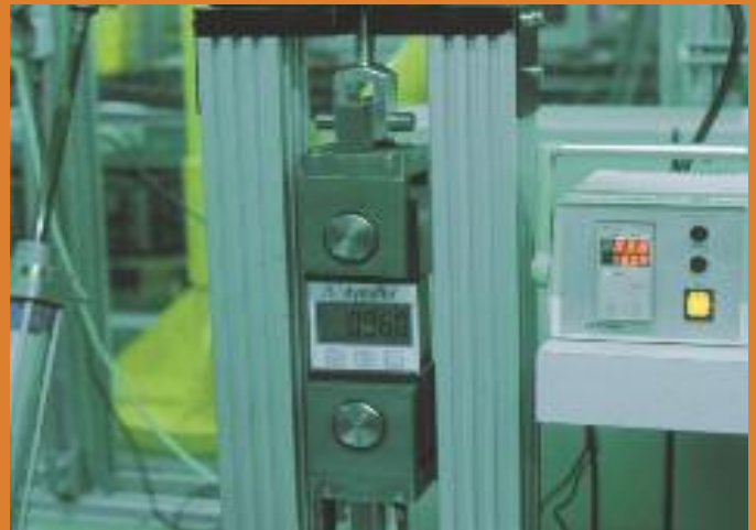
Pictured is a bench test for loads up to 21,755 psi and temperatures up to 482 degrees Fahrenheit.
